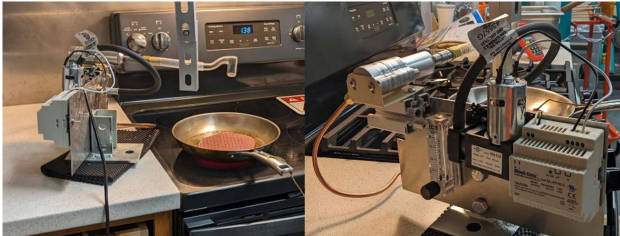
Figure 2. Cooking Emissions Collection System
