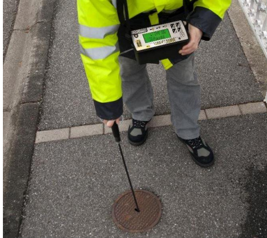
Figure 6: Inspecting sewer with Gazomat Inspectra pump-driven surface sampling detector
