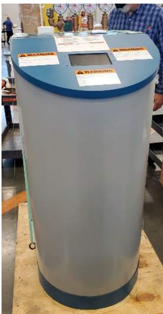
Photo of residential gas heat pump water heater from field trial .
