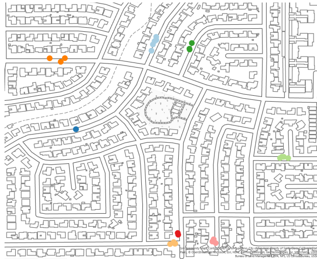
Figure 3: Example of geospatial clustering to associate one or more detections with a source. Each point represents the location where a single plume was detected. Measurements that are clustered together are shown by like colors.
