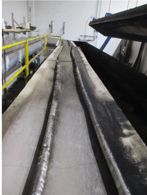
PEXALGAS Metal Tubing 32 x 3 Post-Test
