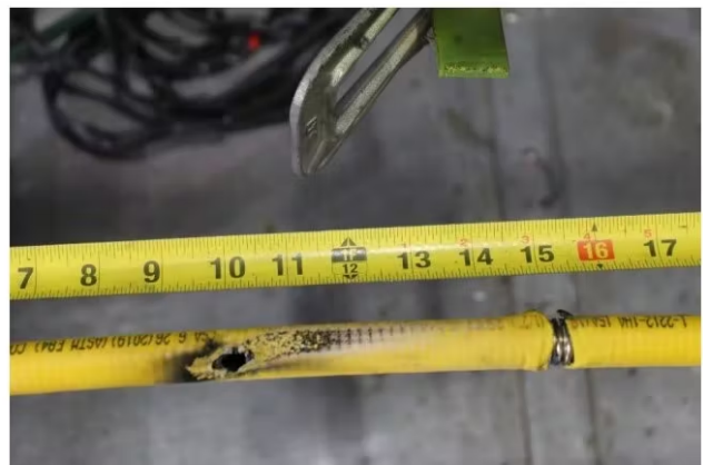
Figure 5 Post Test Visual Assessment – Regular CSST
