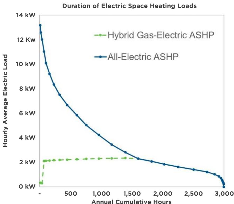
In a hybrid heating system, the heat delivery systems can be programmed to switch from the electric air source heat pump to the natural gas furnace below a balance point temperature.
